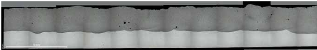
Longitudinal cross section along weld seam over 20 mm distance showing uniform penetration
