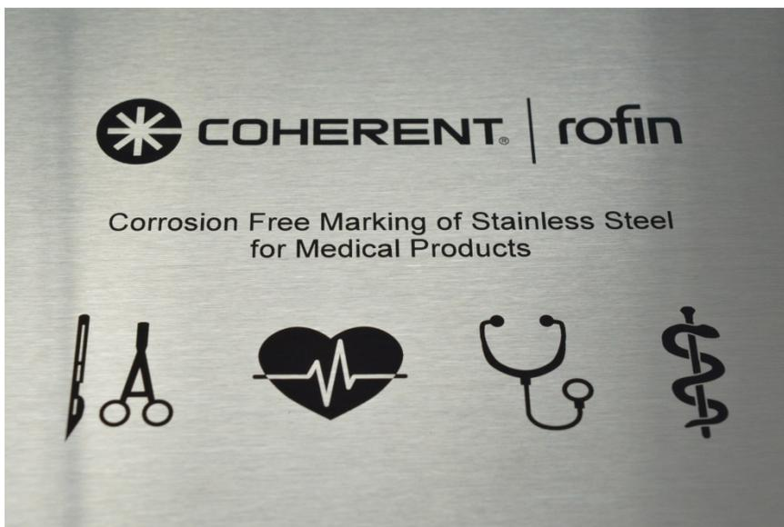
*Figure 2. Some examples of black marks created on 1.4301 steel using a Coherent Rapid NX picosecond laser.*
