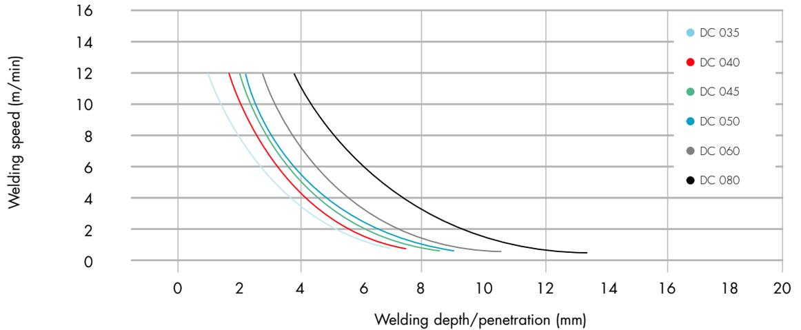
■ You can see clearly there is a uniform increase in the welding depth and speed depending on the laser power. The comparable curve progression makes clear that all lasers are equipped with the same beam quality. Welding depths of up to 12 mm cover the majority of industrial applications.
