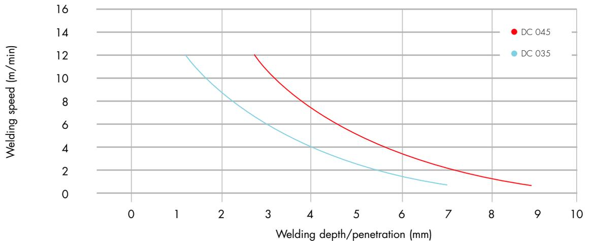
■ Extract from a stainless steel welding curve for 3.5 and 4.5 kW
