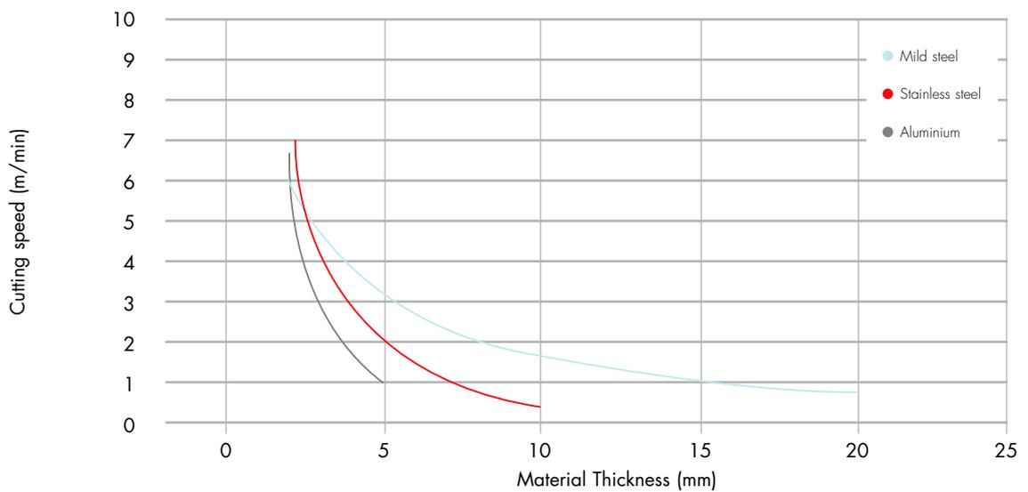
■ This graphic shows the comparison of typical materials (mild steel, stainless steel, aluminium) during the cutting process with a 2.5 kW Slab laser.
