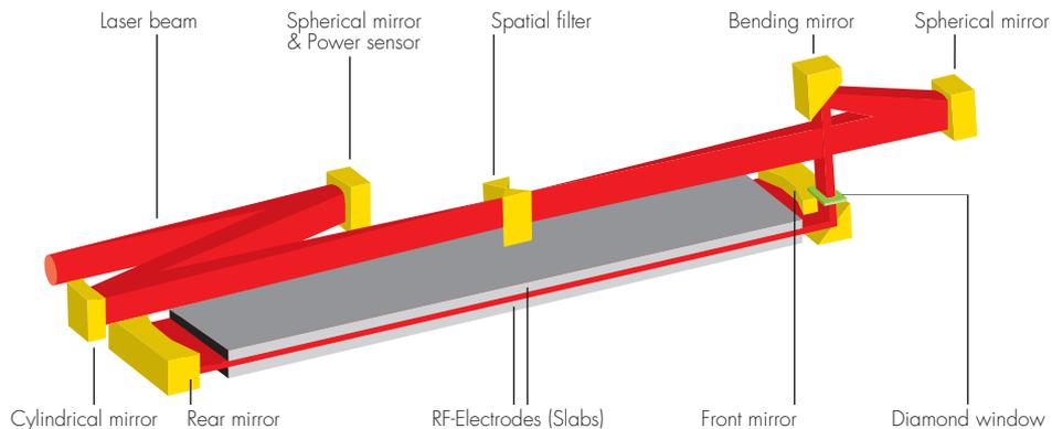
Having left the resonator the laser beam is led through a variety of optics. In order to provide accurate cuts, regardless of direction, water-cooled and reflective beam, components form the originally rectangular beam into a round symmetrical one.
