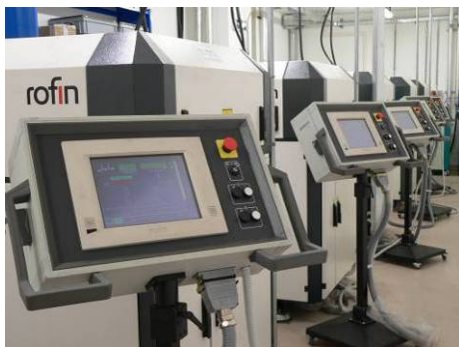
Picture 4: Laser room of the DEKA-VII production with diode pumped solid state lasers from ROFIN
