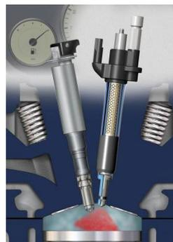
**Picture 5:** Injection valve of Piezo-series
