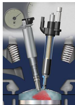
Picture 5: Injection valve of Piezo-series
